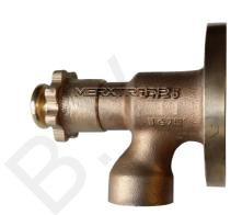
Bronze self closing drain valves are mainly used aboard ships and are spring-loaded with push button for release and locking nut. The button must be pushed to operate the valve. After release of push button, the valve will automatically and instantly close.
