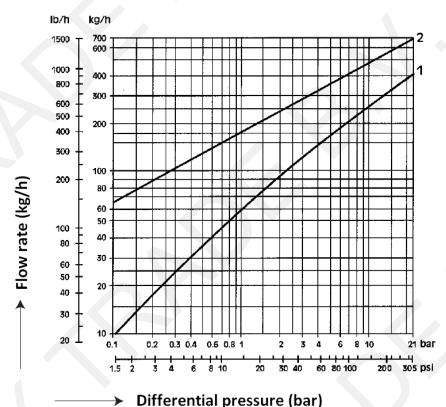
Curve 1: discharge 10 °C below the saturated curve
